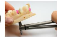
9. Gently push the pliers together. This will pull the analog to a perfect position in the model socket.
