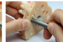
17. Rotate the pliers clockwise until the screw is fully tightened.
