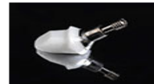
materially bonding of Ti and ZrO 2
