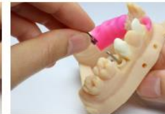
3. Stick the pin through the bottom of the printed model and screw it into the bottom of the analog.
