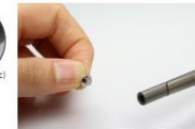
14. Place the fixation screw in the socket wrench of the Elos Accurate Pliers.
