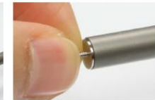
15. The socket wrench has a magnetic feature which will keep the fixation screw securely in place.
